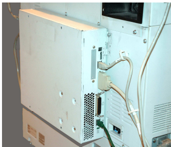
A typical print controller attached to the back of a digital copier.
