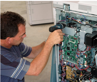
John Juntunen extracts the hard drive from a digital copier
